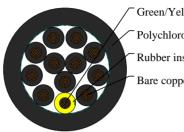
Green/Yellow wire Polychloroprene rubber outer jacket Rubber insulation Bare copper conductor
